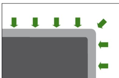
Compressive stresses in the CVD coating caused by mechanical post-treatment
