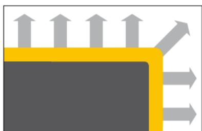
Tensile stresses/risk of fractures in the CVD coating
