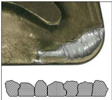
Conventional aluminium oxide – high level of crater wear due to random structural arrangement
