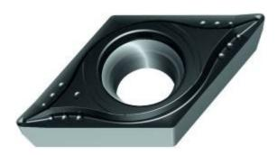
Caption: The PVD aluminium oxide coating on the new Tiger·tec® Silver WSM10S, WSM20S and WSM30S cutting tool materials protects the carbide against heat loading. This heat shield enables longer tool life and higher cutting speeds to be achieved – particularly when machining stainless materials (ISO M) and heat-resistant alloys (ISO S).
