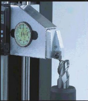
Precise measurement by 2D switch. Index at fixture spindle (optional).
