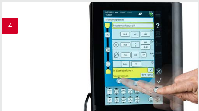
4 Simple Drag & Drop tasks and saved ISO tolerance tables make it very easy to create measuring programs.
