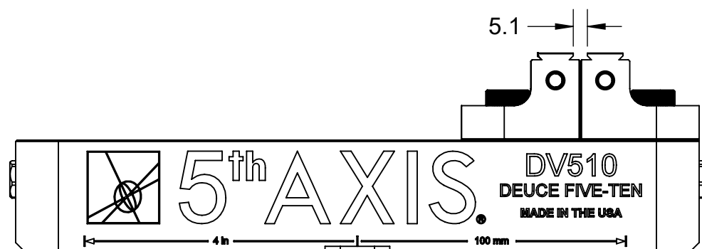
FORWARD JAWS (MINIMUM CLAMPING RANGE) FIXED JAW CONFIGURATION
