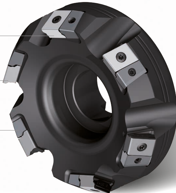
Heavy-duty M3016 cutter, 160 mm diameter, \kappa = 60^\circ with LNMX201012 system indexable insert.
