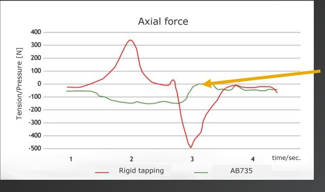
Low axial force compared to rigid clamping
