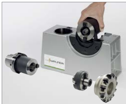
5. Insert the extension into the insert collar
