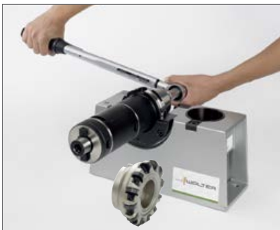
10. Tighten using a torque wrench
