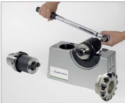
7. Tighten using a torque wrench
