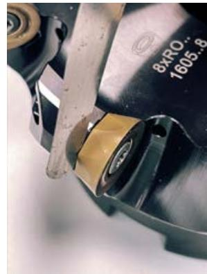
④ Check that the indexable insert is securely fitted
